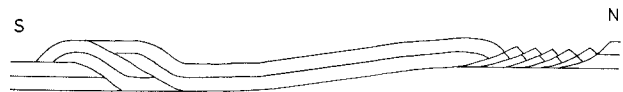
Fig. 14. Schematic cross-section showing how extensional geometries in the Little Beauty Syncline (cf. Holcombe et al. 1991) can transfer into thrust geometries in the Rosebud Syncline.
